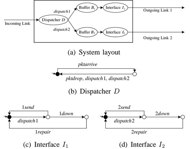
Fig. 2. Illustrative example 2: Network switching system
