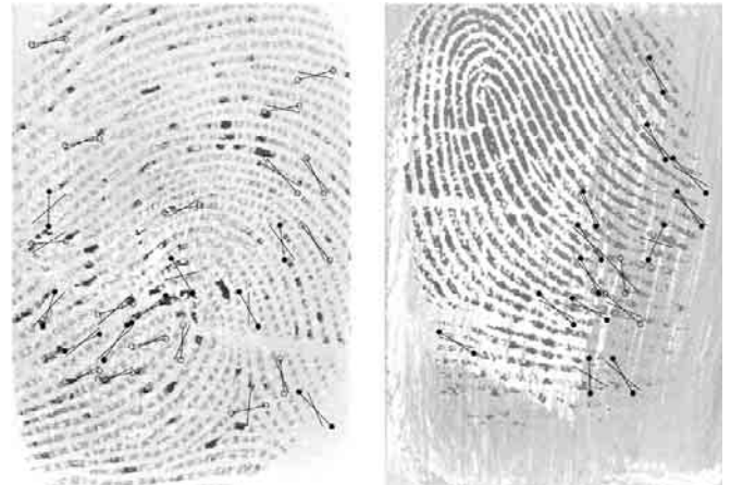
Fig. 14. Two real fingerprints and orientation estimates where visible difference can be found. Unmarked lines and lines marked by circles and dots represent \Theta_{QA}^\Gamma , \Theta_1^\Gamma , and \Theta_r^\Gamma , respectively.
