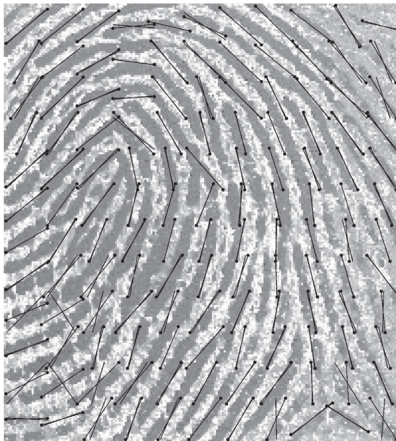
Fig. 6. Estimated local orientations of the bad quality fingerprint in Fig. 5. Short lines marked by dot are for the proposed operator and unmarked ones are for the \nabla G operator. Both operators are of size 5 \times 5 .
