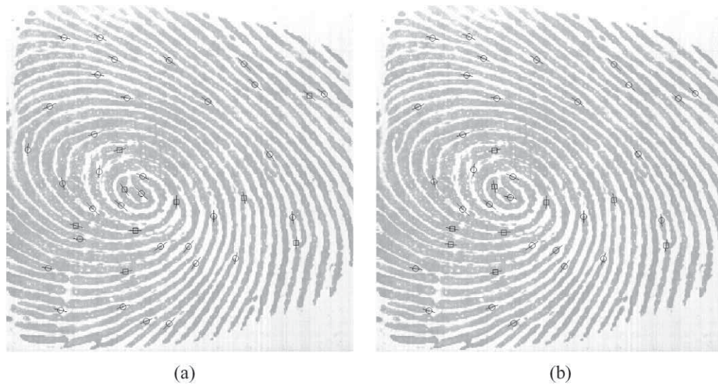
Fig. 9. Examples of detected minutiae with fixed step 1(a) and with adaptive step (b) for an image captured with Veridicom CMOS sensor.
