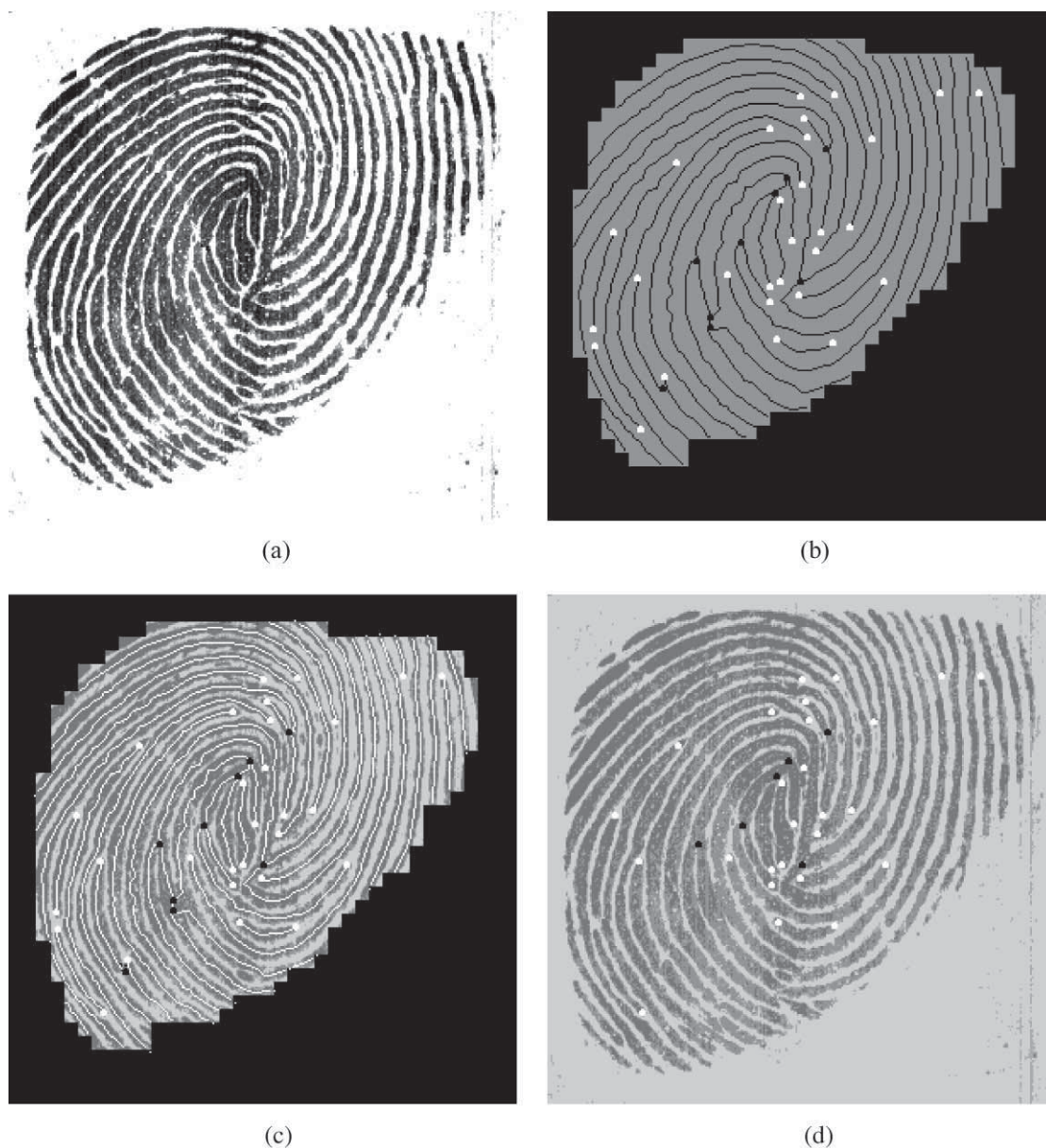
Fig. 8. A sample fingerprint (a), the detected skeleton ridges and minutiae before the post processing (b), (c) and after the post processing (d).
