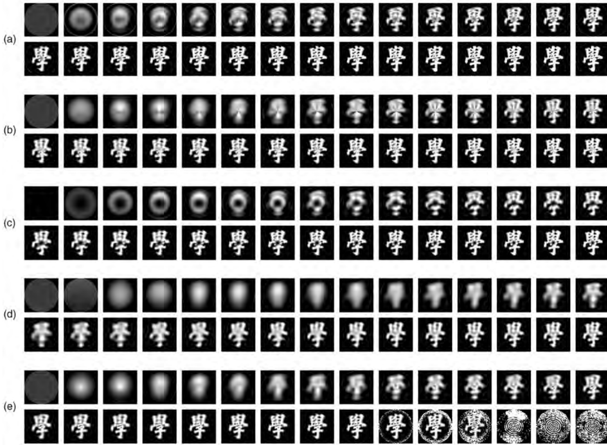
Fig. 3. Some samples of reconstructed images. K = 0, 1, \dots, 29 . (a) Polar complex exponential transform, (b) polar cosine transform, (c) polar sine transform, (d) Zernike moments, and (e) pseudo-Zernike moments.
