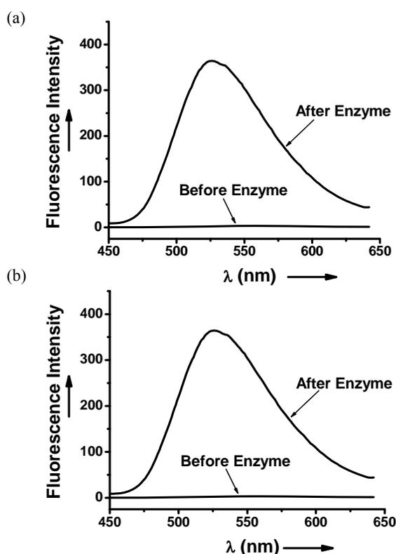
Figure 1. Fluorescent measurement of MAO enzymatic reactions. Emission spectrum of MAO-HPQ **1** (200 μM) upon treatment with MAO A (a) and MAO B (b) in Tris-HCl buffer (100 mM, pH 7.90). Enzyme concentration: 10 μg/ml. Excitation wavelength: 360 nm, Emission wavelength: 530 nm.
