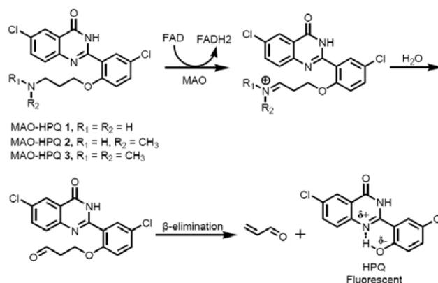
Scheme 1. Fluorescent detection of MAO activity by oxidative deamination of HPQ derivatives and subsequent  $\beta$ -elimination.
