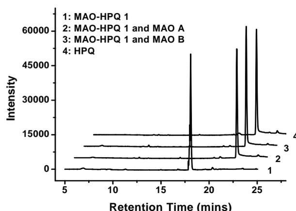
Figure 2. HPLC analysis of enzymatic reaction of MAO-HPQ **1** with MAO isozymes. Absorbance wavelength: 360 nm
