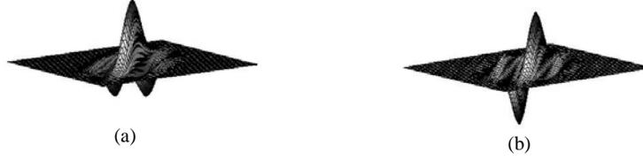
Fig. 1 (a) The real part and (b) the imaginary part of a Gabor filter
