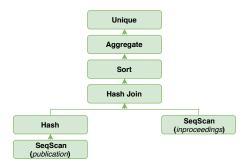
Figure 4: A physical operator tree (i.e., QEP).
