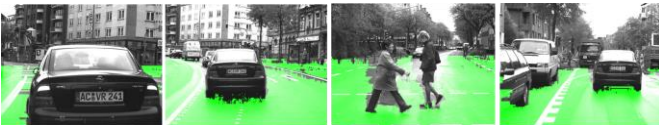
Fig. 10. Examples of detection results of proposed algorithm for scenarios where the vicinity of the vehicle is filled with crowded objects.
