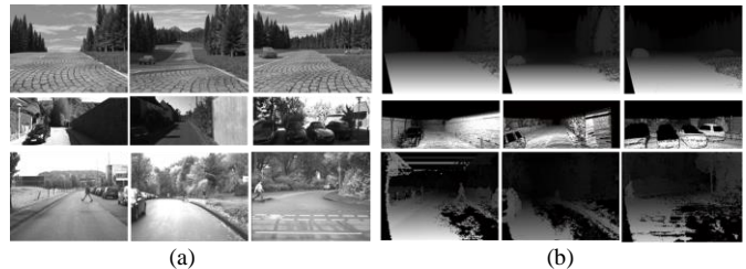
Fig. 6. Samples of (a) left images of the stereo pairs from the enpeda dataset (first row), the KITTI dataset (second row), and the Daimler dataset (third row) and (b) their corresponding disparity maps for the three benchmarks used in our experiments. The contrast is enhanced for better visualization. The disparity maps serve as the inputs.
