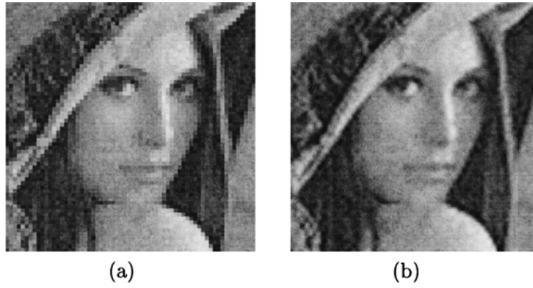
Figure 3. Lena image (a) zero order hold expanded and (b) cubic spline interpolated.
