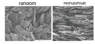
A team of scientists led by Nanyang Assistant Professor Hortense Le Ferrand, Nanyang Technological University's School of Mechanical and Aerospace Engineering, used magnetic fields to align and orient microscopic particles of BN, which can direct heat away from the source to prevent overheating. The study "Microstructured BN composites with internally engineered highly thermally conductive paths for 3D electronic packaging" can be found in Advanced Materials.
