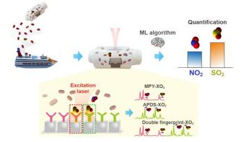
An overview of how the SERS chip detects NO2 and SO2 in vehicle exhaust. Credit: NTU Singapore.
