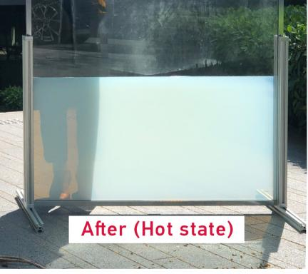
At the same time, the high heat capacity of water allows a large amount of thermal energy to be stored instead of getting transferred through the glass and into the building during the daytime when it is hot.
