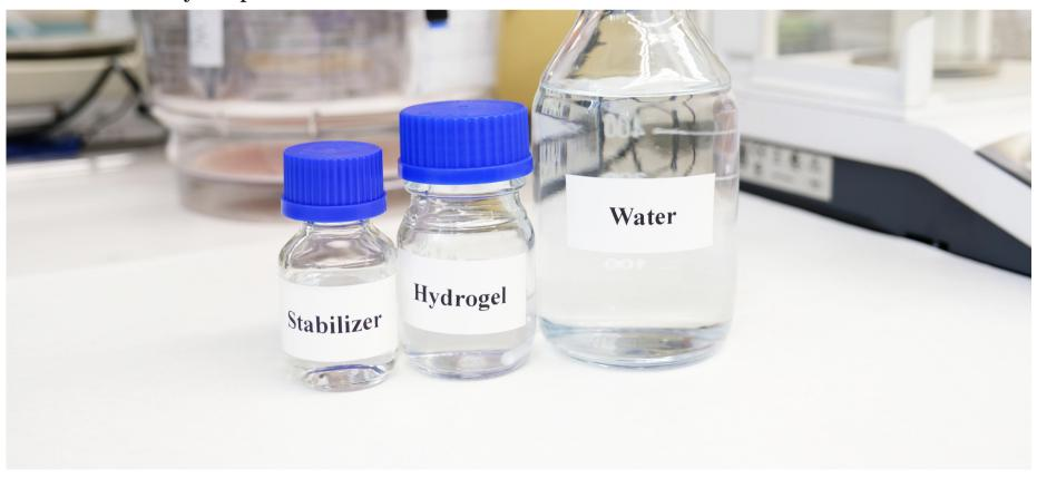
The liquid mixture used to create the smart window is made from micro-hydrogel, water and a stabiliser. Photo: Nanyang Technological University
