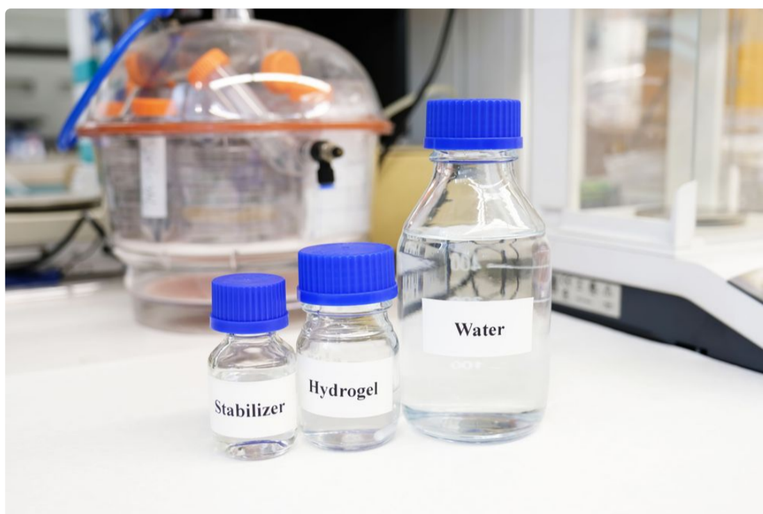
The liquid mixture used to create the smart window is made from micro-hydrogel, water and a stabiliser. — Nanyang Technological University pic via TODAY
