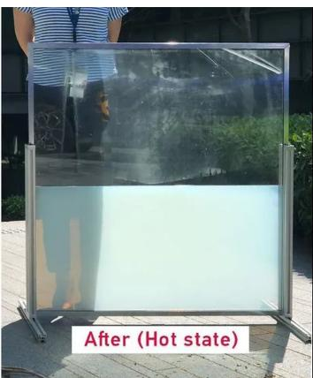
The smart window turns opaque when exposed to heat, thus blocking sunlight, and, when cool, returns to its original 'clear' state. (Photo: Nanyang Technological University)
