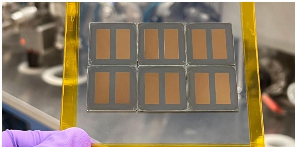
1-cm<sup>2</sup> prototype perovskite solar cells fabricated with NTU team's selective template growth (STG) method
