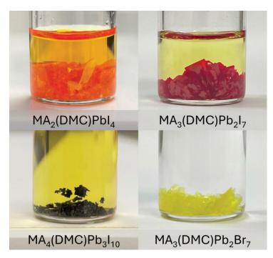
Semiconductor materials known as 2D halide perovskites can be used in devices such as solar cells and light-emitting diodes. Scientists led by Assoc Prof Nripan Mathews of NTU's School of Materials Science and Engineering have synthesized four unique types of 2D halide perovskites.
