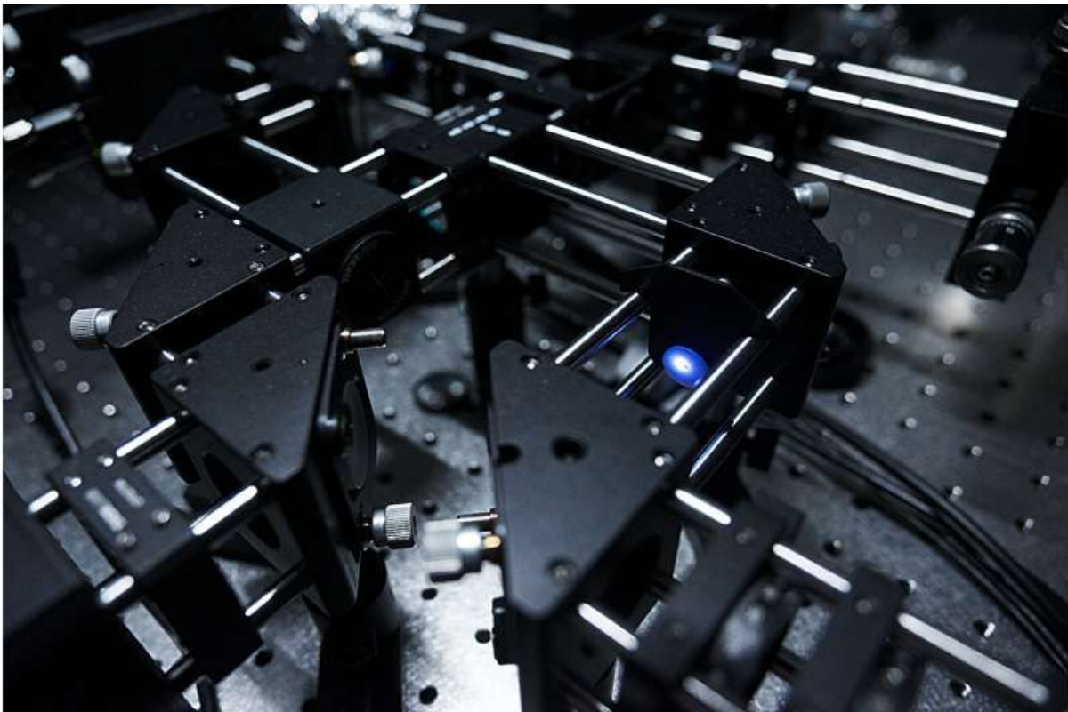
A blue laser set-up for producing entangled pairs of photons in NTU Singapore’s experiments. Credit score: NTU Singapore
