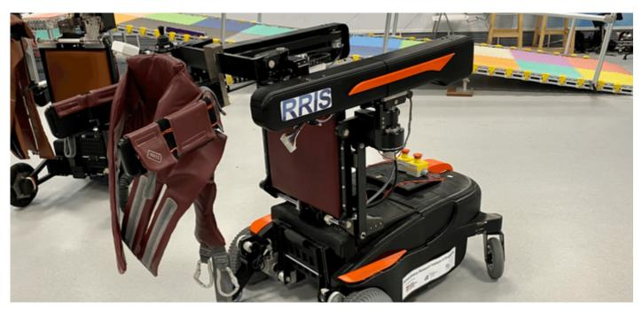
Developed by NTU Singapore and TTSH, MRBA is a wearable assistive robot that can detect and prevent a fall before it happens, reducing the user's risk of sustaining injuries | Photo source NTU Singapore
