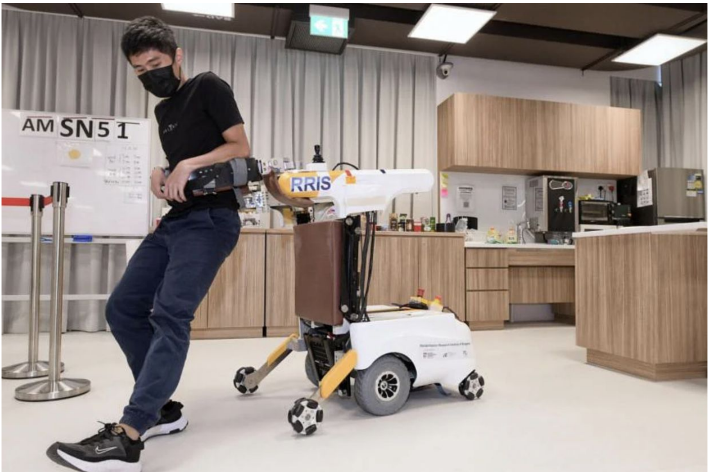
The Mobile Robotic Balance Assistant has a harness, which the user wears on his hips, that can counter falls and imbalances. — NG SOR LUAN/The Straits Times/ANN
