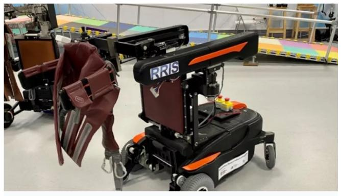
Developed by NTU Singapore and TTSH, MRBA is a wearable assistive robot that can detect and prevent a fall before it happens, reducing the user's risk of sustaining injuries - NTU Singapore
