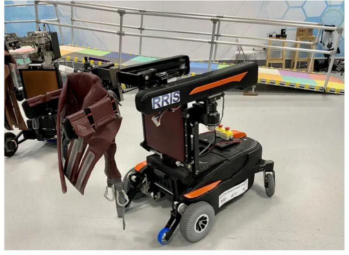
Developed by NTU Singapore and TTSH, MRBA is a wearable assistive robot that can detect and prevent a fall before it happens, reducing the user's risk of sustaining injuries. NTU SINGAPORE
