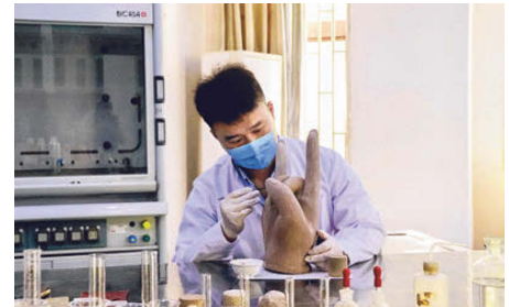
Dr Yang Yang restoring (below) a Buddha hand from the Dazu Rock Carvings, a Unesco World Heritage Site in China, with the biocement in Chongqing University in China. The team member and former NTU PhD student and research associate at the Centre for Urban Solutions is currently a postdoctoral fellow at Chongqing University. The biocement solution is colourless, allowing restoration works to maintain the carving's original colour.
