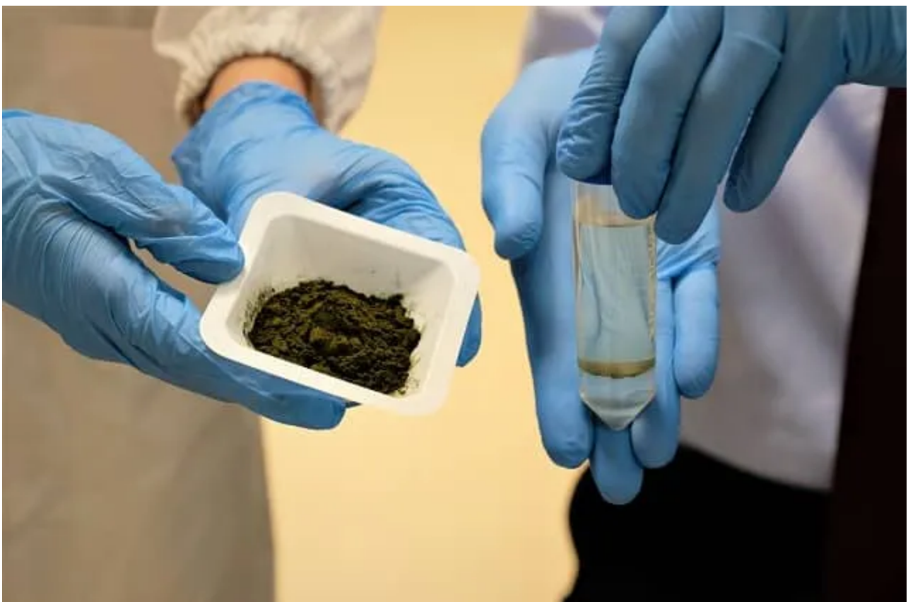
Powdered microalgae that has been washed, dried, and treated with methanol by NTU researchers, with a vial of oil produced from microalgae on the right
