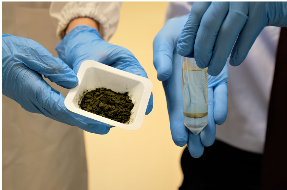
Powdered microalgae that has been washed, dried, and treated with methanol, with a vial of oil produced from microalgae on the right. (Image: NTU Singapore)
