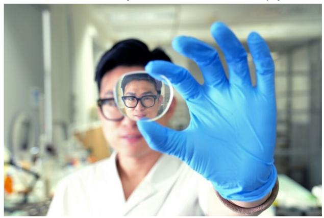
That transparent film comprises two layers – one consisting of silicon dioxide, the other of titanium dioxide – and it's placed on the plastic through a pulsed laser deposition process. The latter involves using a laser to vaporize each of the two-layer materials within a vacuum chamber. As the vaporized silicon dioxide and titanium dioxide rise upwards, they're finely deposited on the plastic substrate, which is located at the top of the chamber.
