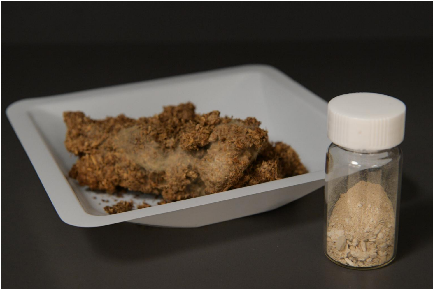
The plant-based emulsifier (in bottle) is produced by fermenting spent barley grains (background), a main byproduct of the brewing industry. ST PHOTO: NG SOR LUAN
