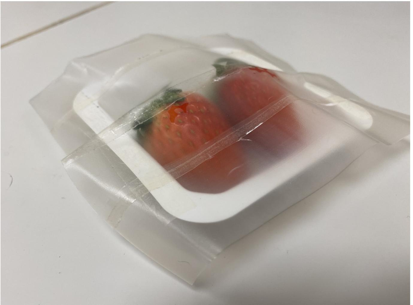
*In an experiment, strawberries that were wrapped in the NTU-Harvard University-developed packaging stayed fresh for seven days before developing mould, compared to counterparts that were kept in mainstream fruit plastic boxes, which stayed fresh for four days. Credit: Nanyang Technological University*
