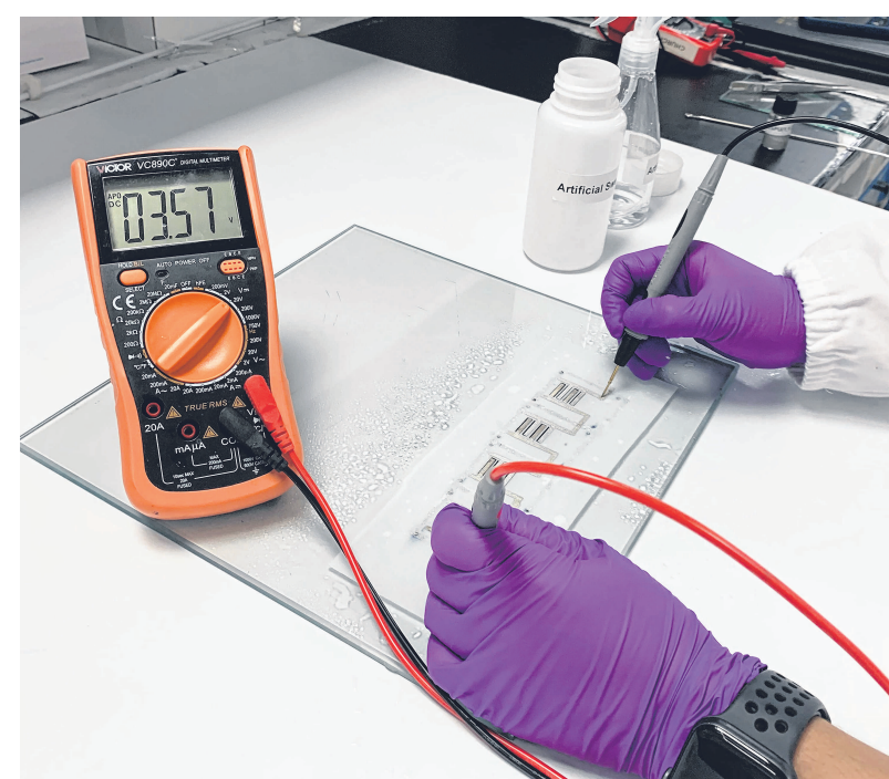
After being sprayed with artificial sweat, the battery generated a voltage of 3.57V. Each battery is 2cm by 2cm, about the size of a small postage stamp.
