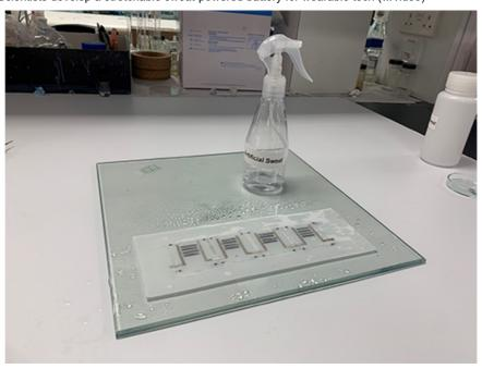
To demonstrate its potential use when it becomes incorporated in wearable biosensors and other electronic devices, the team of scientists at NTU tested their device with artificial human sweat.
