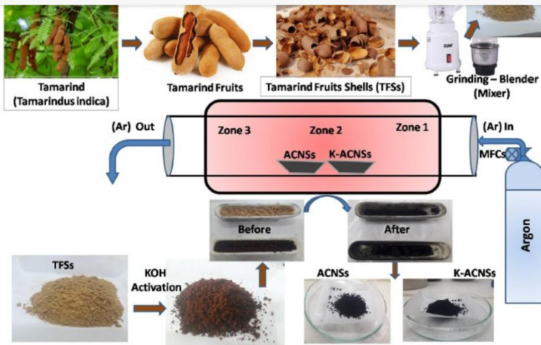
A representation of the experimental process, as well as photographs of the tamarind shell at every step. *Image: NTU Singapore*
