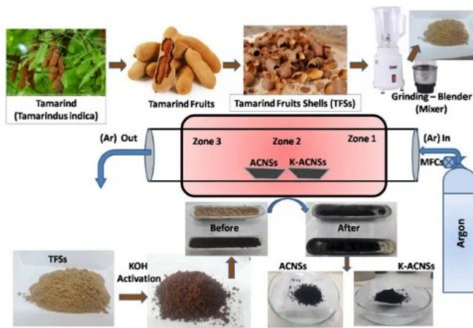
A representation of the experimental process, as well as photographs of the tamarind shell at every step. Image Credit: Nanyang Technological University.
