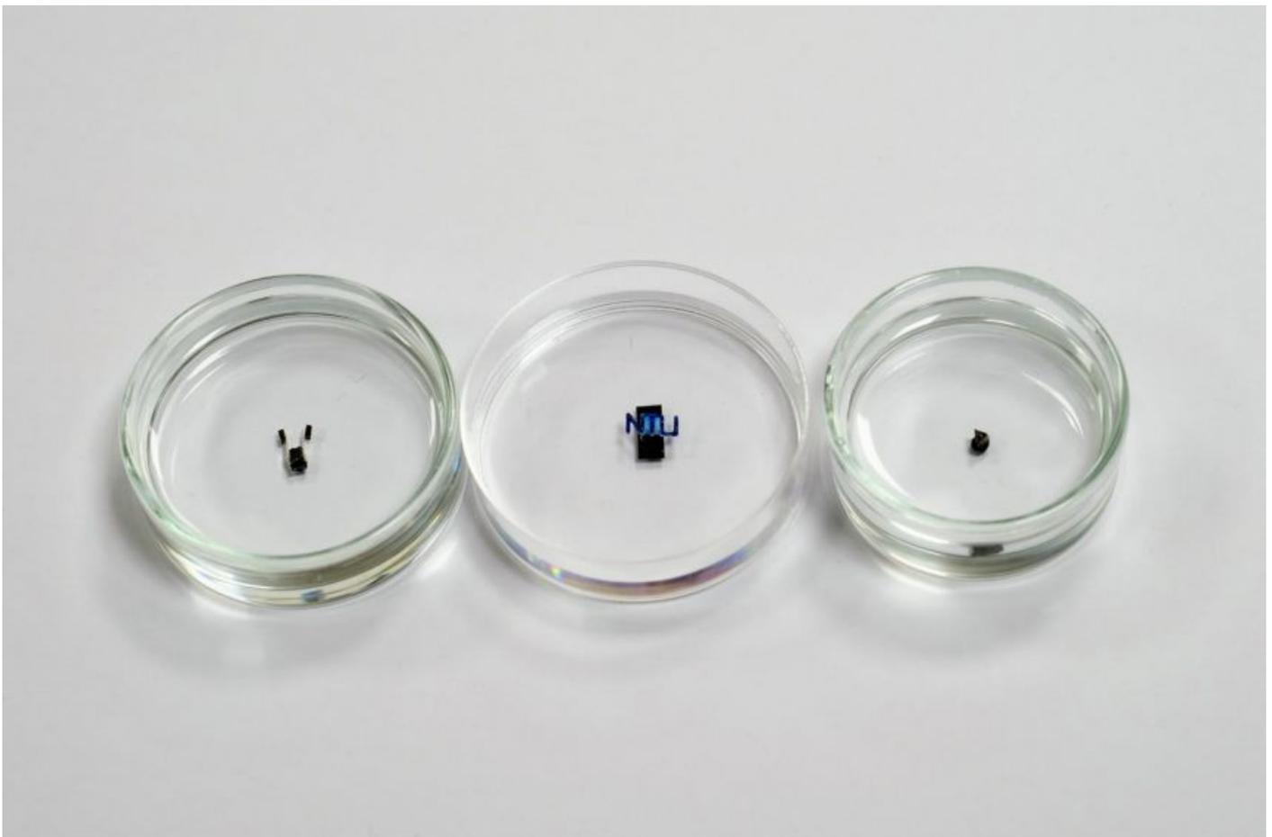
The miniature robots were created by embedding small magnetic particles into materials that are harmless to humans. — Photos: NTU SINGAPORE
