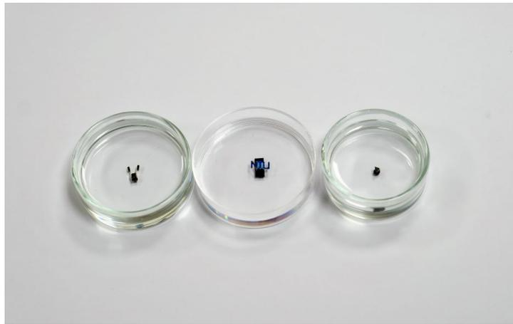
The NTU millimetre-sized robots measure about the size of a grain of rice and can be controlled using magnetic fields (Image: NTU Singapore)
