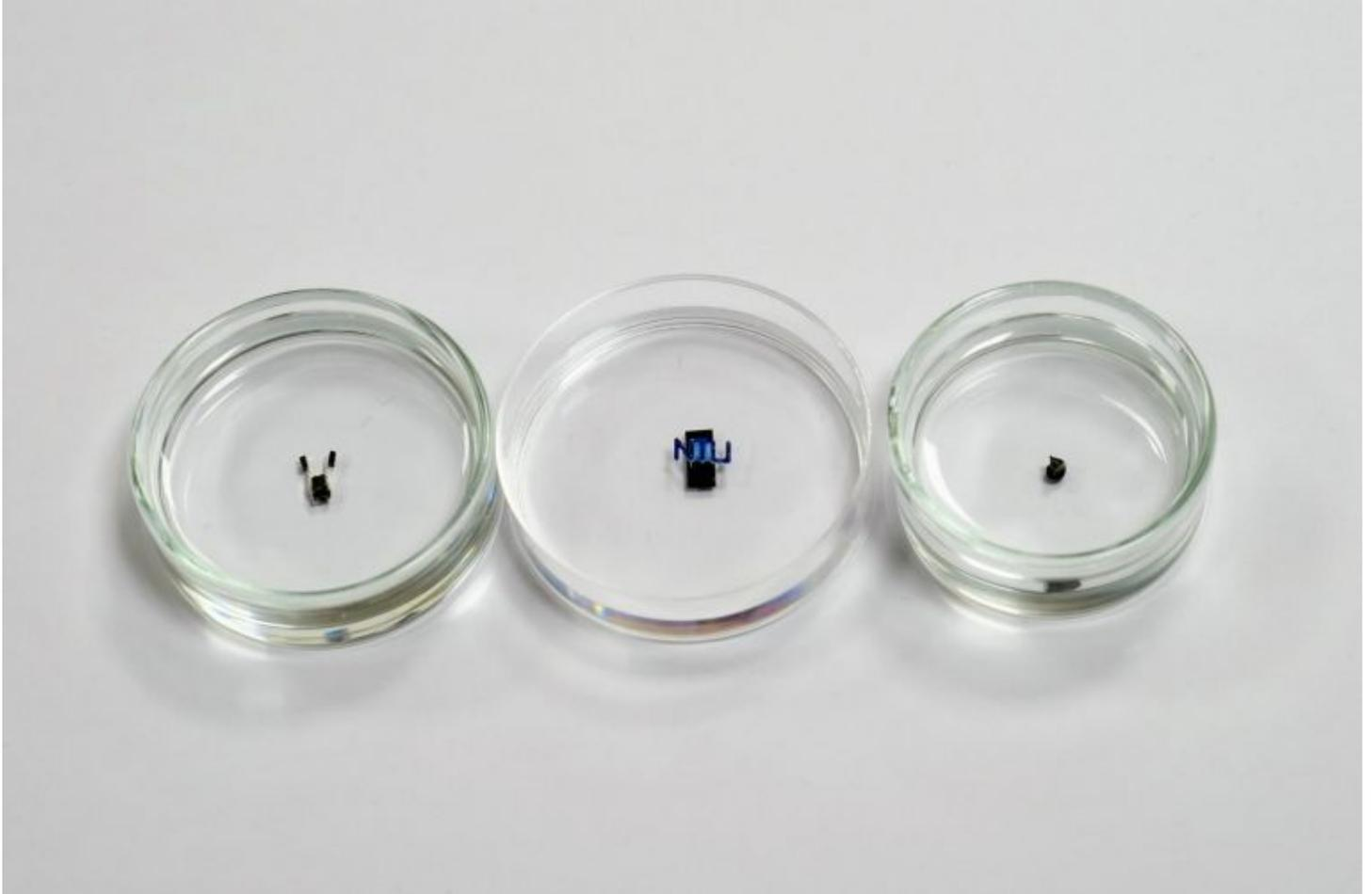
The miniature robots were created by embedding small magnetic particles into materials that are harmless to humans. PHOTO: NTU SINGAPORE
