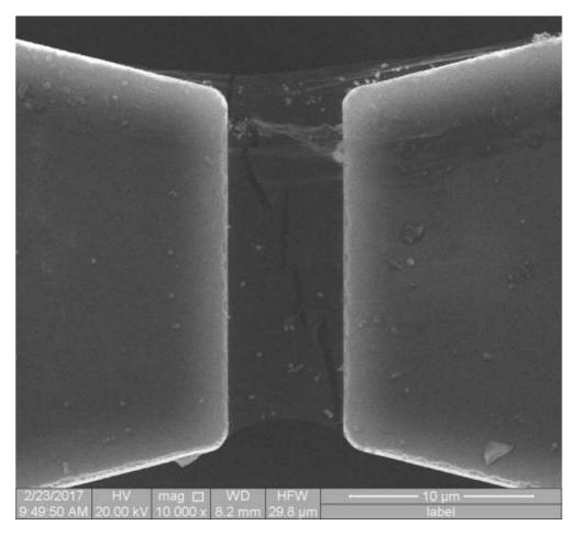
A scanning electron microscope image shows branched cracks in a single crystal of 2D hexagonal boron nitride (h-BN). Experiments and computational modelling by Rice University and Nanyang Technological University showed h-BN lattice asymmetry allows cracks to follow branching paths, which effectively toughens the 2D material by making it more difficult for cracks to propagate. Credit: J. Lou/Rice University
