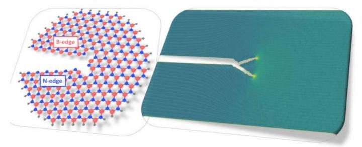
Computational simulations at Nanyang Technological University in Singapore helped explain the unexpected fracture toughness of 2D hexagonal boron nitride. The material's intrinsic toughness arises from slight asymmetries in its atomic structure (left), which produce a permanent tendency for moving cracks to follow branched paths (right). Credit: H. Gao/NTU
