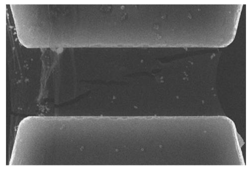
A scanning electron microscope image shows branched cracks in a single crystal of 2D hexagonal boron nitride (h-BN). Experiments and computational modelling by Rice University and Nanyang Technological University showed h-BN lattice asymmetry allows cracks to follow branching paths, which effectively toughens the 2D material by making it more difficult for cracks to propagate. (Image courtesy of J. Lou/Rice University)
