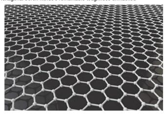
In both graphene and hexagonal boron nitride (h-BN) atoms, atoms are arranged in a flat lattice of interconnecting hexagons. In graphene, all the atoms are carbon. In h-BN each hexagon contains three nitrogen and three boron atoms. (Image: Rice University)
