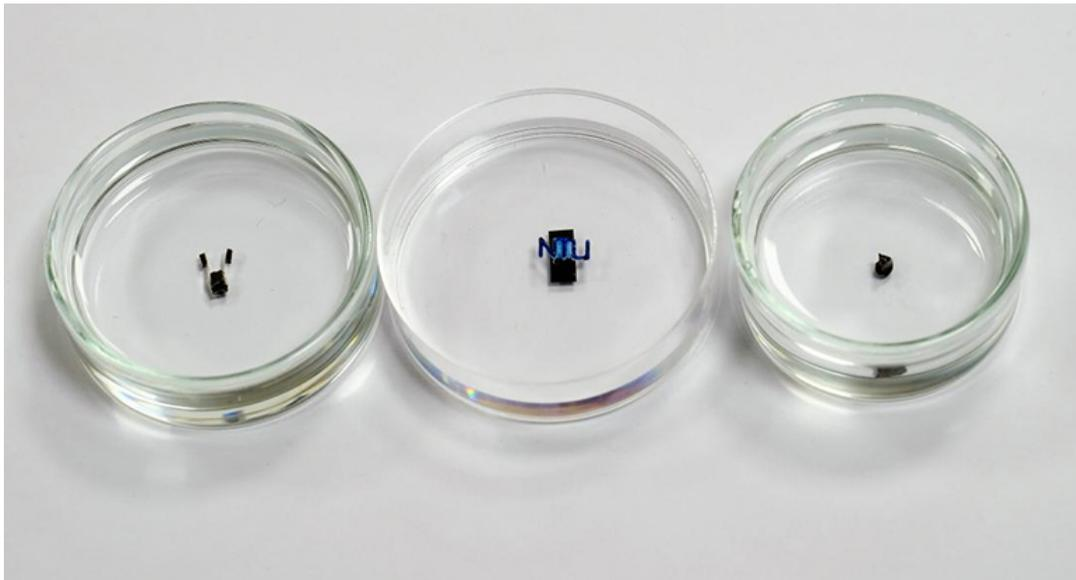
Researchers at Nanyang Technological University, Singapore have developed miniature robots that are highly maneuverable, and can rapidly move in six degrees of freedom. These tiny devices are magnetic and can be controlled using an electromagnetic coil system that precisely manipulates the direction and strength of magnetic fields. The researchers hope that their technology could pave the way for tiny surgical robots that could access difficult to reach areas in the body, such as the brain.
