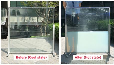
The newly developed 'liquid windows' show significantly lower levels of heat permeability into buildings, and also offer better noise reduction that other window types. Image credit: Nanyang Technological University
