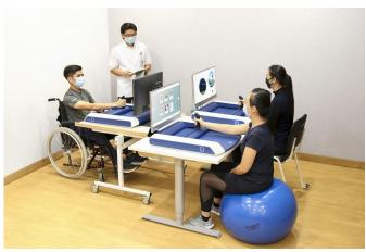
The H-Man is a portable arm rehabilitation robot, weighing only 14kg that post-stroke patients could use for rehabilitation therapy at home or in community-based
