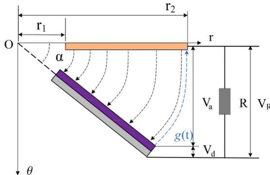
Fig. 3. Schematic of tribo-pair with non-parallel configuration.
