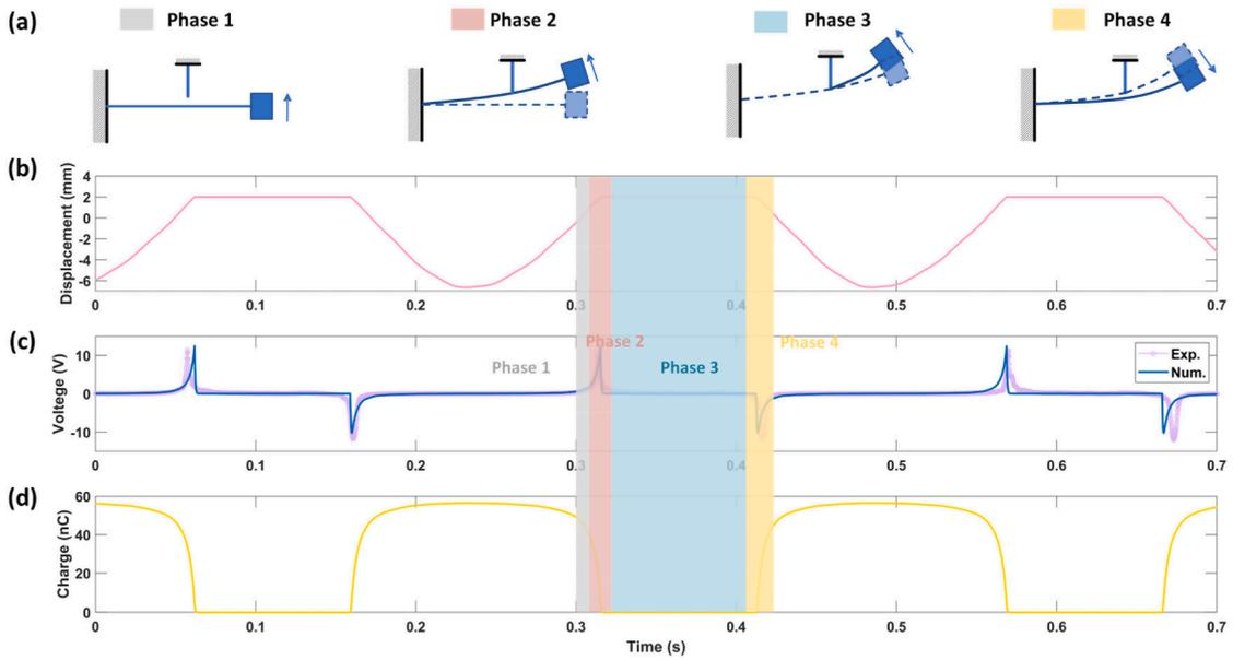
Fig. 7. Simulated displacements, voltage outputs, and charges at different phases of the impact-engaged galloping vibration process.
