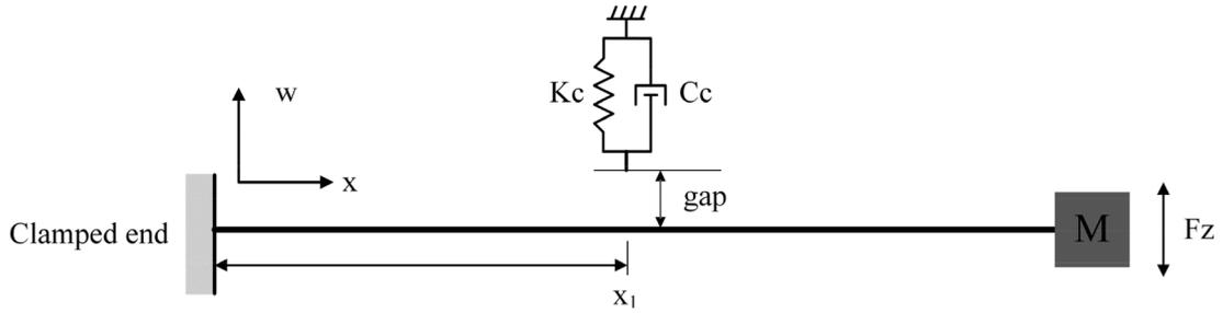
Fig. 2. Schematic diagram showing simplified model of GTEH.
