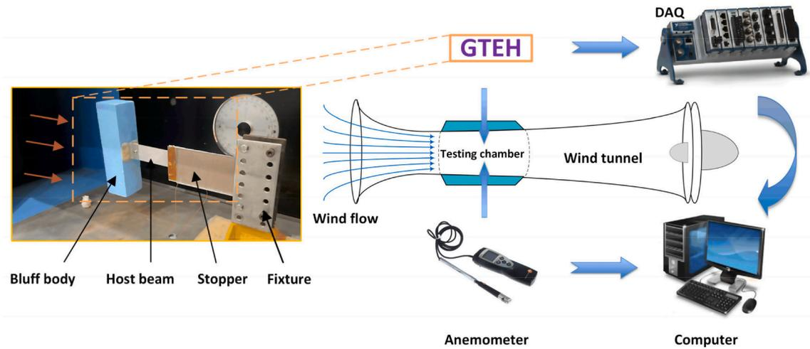
Fig. 4. Experimental setup for testing the proposed GTEH.
