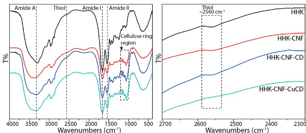
**Figure 2.** Fourier transform infrared spectroscopy (FTIR) spectra of HHK, HHK-CNF, HHK-CNF-CD, and HHK-CNF-CuCD samples.
