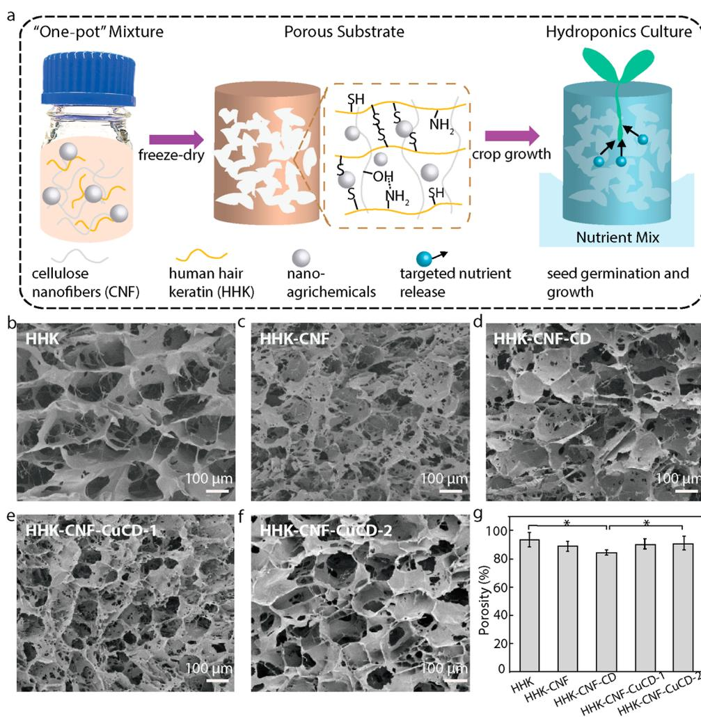
**Figure 1.** (a) Schematic illustration of the fabrication process of HHK-CNF-agriche-mical substrates via a freeze-drying method and their potential use in hydroponics. Morphologies of HHK (b), HHK-CNF (c), HHK-CNF-CD (d), HHK-CNF-CuCD-1 (e), and HHK-CNF-CuCD-2 (f) under SEM. The porosity of all these samples was calculated using a liquid displacement test (g), \* $p < 0.05$  ( $n=3$ ).
