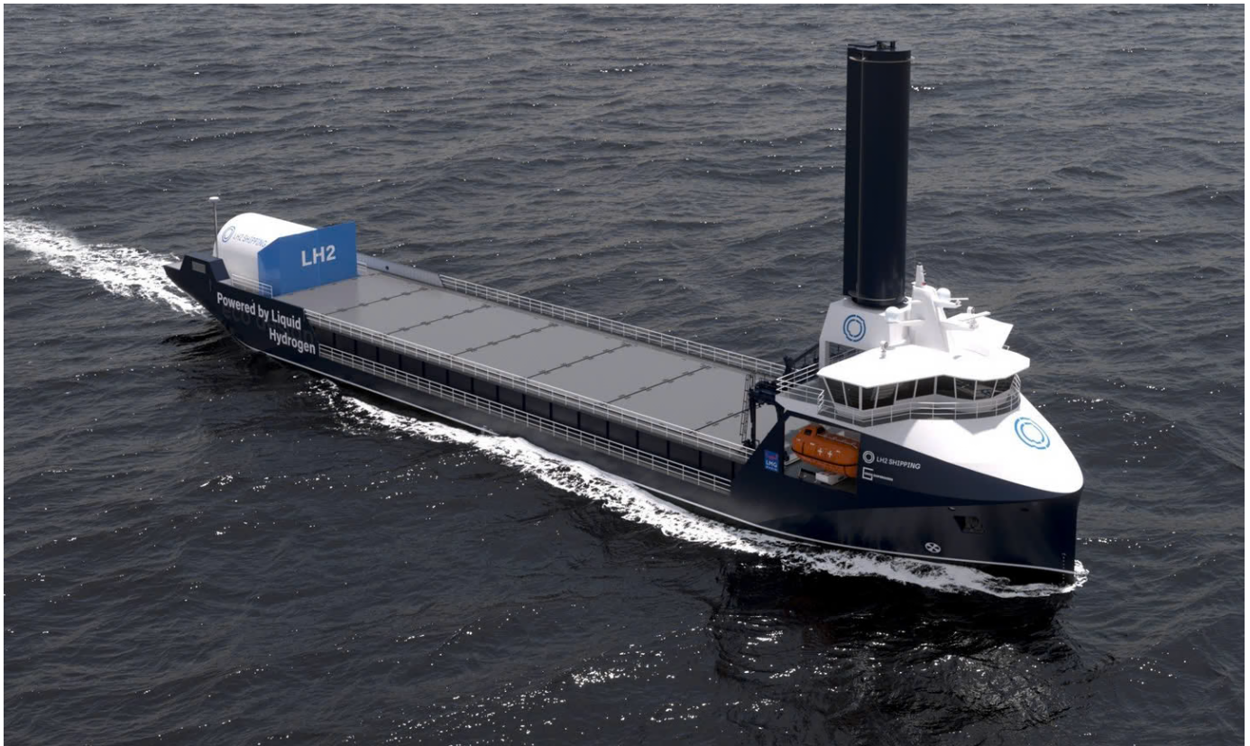
The Hydrobulk ship from LH2 Shipping, powered by liquid hydrogen (LH2). Photo: LH2 Shipping/Sigve Hoff Larsen.
