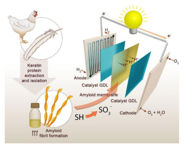
Representation of the components of the fuel cell. In the center is the membrane made of keratin. To the left and right of the membrane is a catalyst. In the outer layer is the anode on one side and the cathode on the other.© Daily Galaxy NZ
