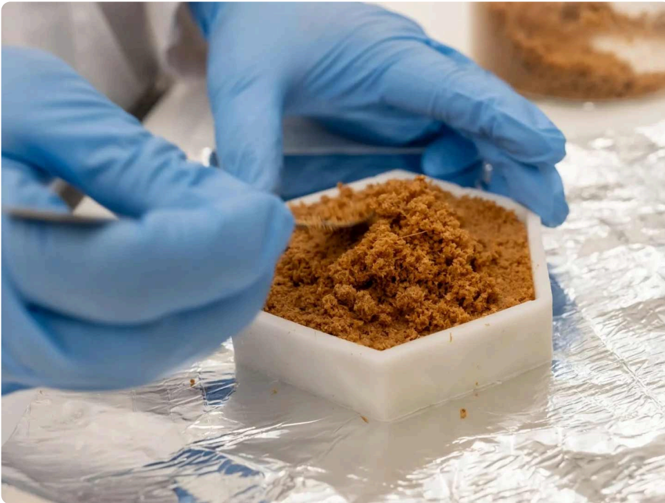
RESEARCHERS MIX A COMBINATION OF MYCELIUM AND BAMBOO SHAVINGS IN THE HEXAGONAL MOLD. PHOTO COURTESY OF NANYANG TECHNOLOGICAL UNIVERSITY SINGAPORE
