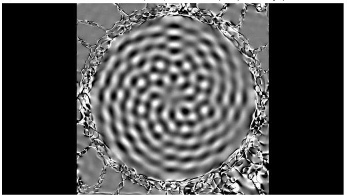
The image shows how water swirls in complex patterns produced from waves generated by a ring-shaped plastic structure in a water tank. The image was generated while analyzing how water moves up and down in the patterns. Credit: Henan University
