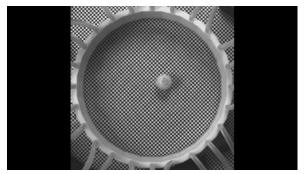
The researchers were able to get a ping pong ball floating in a water tank to spin about its center and move along a fixed circular path by using waves they generated with a ring-shaped plastic structure. Credit: Henan University
