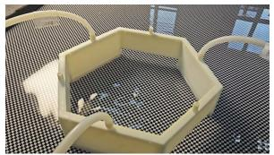
A hexagon-shaped plastic structure was used to generate waves that merged to form complex patterns on the water surface in a tank for an experiment co-led by Nanyang Technological University, Singapore. These patterns drew in and trapped a floating foam ball. Credit: Henan University
