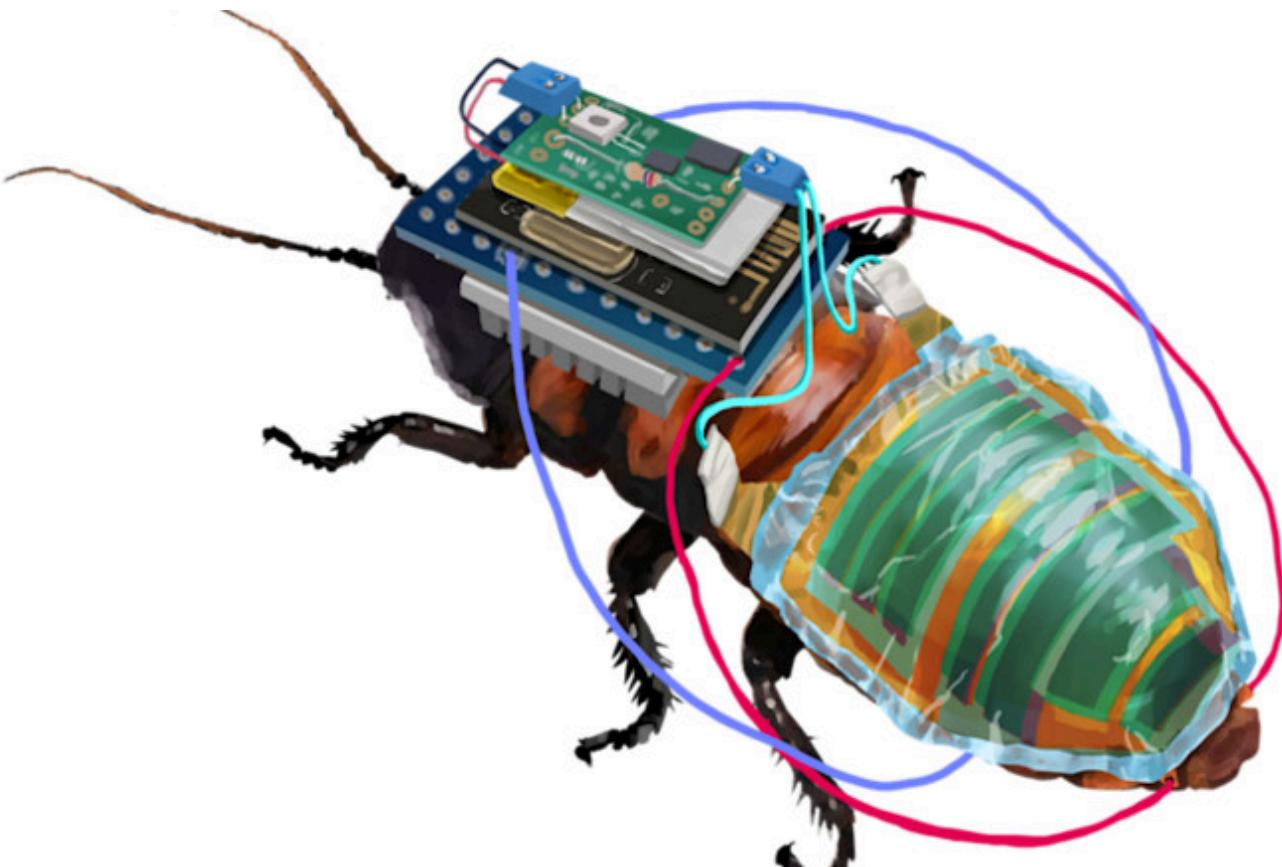
Researchers at RIKEN, Japan have created remote controlled cyborg cockroaches, equipped with a tiny wireless control module that is powered by a rechargeable battery attached to a solar cell. (Credit: RIKEN)
