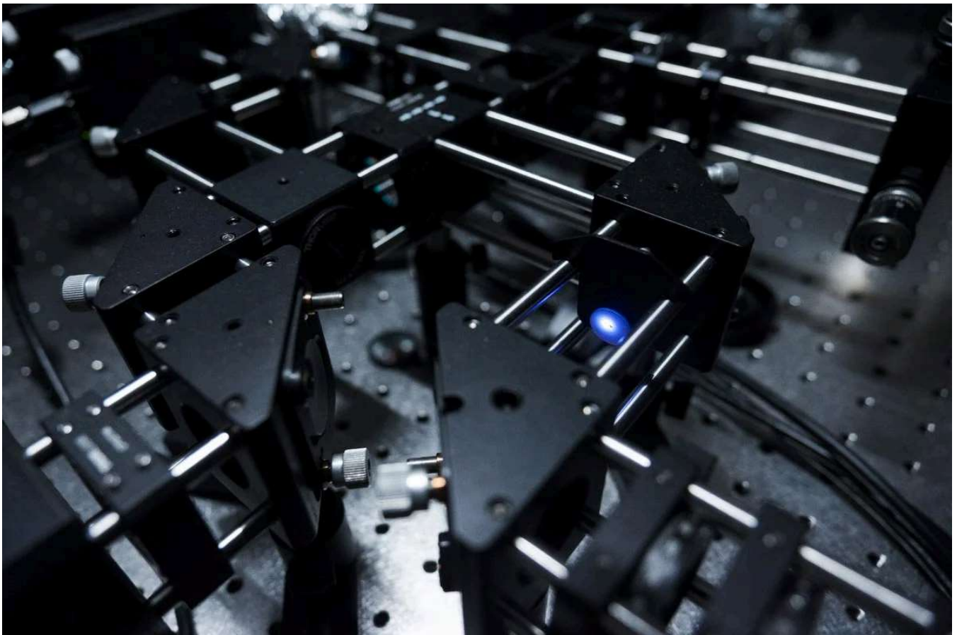
A blue laser setup for generating entangled pairs of photons in NTU Singapore’s experiments. Credit: NTU Singapore
