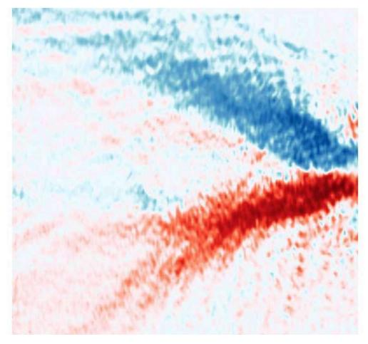
An electric field applied to a microcavity structure caused polaritons with different spins to move away from one another in opposite directions. This is visualized here by a spectrometer, with red polaritons spinning in one way separated from blue polaritons spinning the other way after they moved apart. Credit: Nanyang Technological University, Singapore
